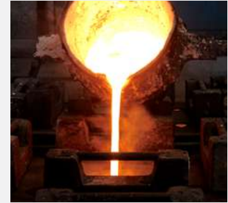
casting the escutcheon plate
